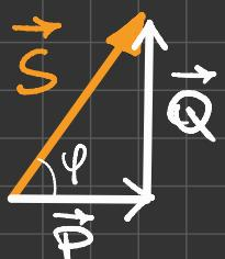
$$P = S \cos \varphi = 3 \sqrt{V_2} I_f \cos \varphi = 3 E I_f \cos \varphi = \sqrt{3} \sqrt{I_f} \cos \varphi$$
