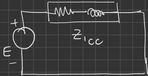
$$\bar{Z}_{1cc} = R_{1cc} + jX_{1cc} = Z_{1cc} \angle \varphi_{cc}$$
